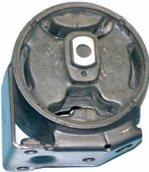
Figure 2-1. Engine mount of a Volkswagen Golf II, 1985.
